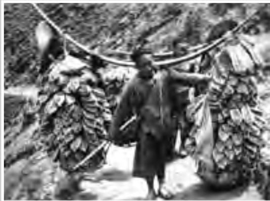
The natural spring of split bamboo carrying poles eased worker's loads such as this one of woven straw shoes, the most common footwear in Southern China.
